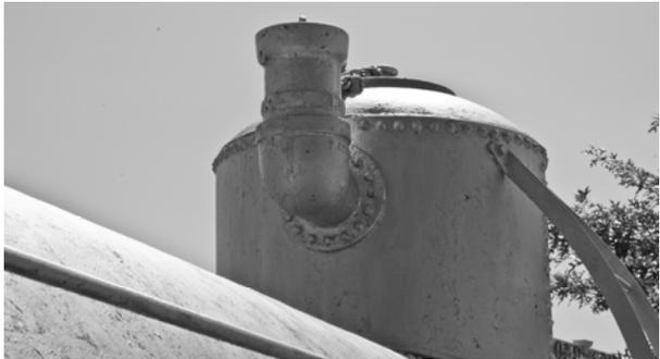
The flange of the vent is tightly riveted to the side of the dome. The rivets are much smaller in diameter than those used on the side and ends of the car too.
