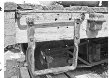
Also when the steps and grabs were added to the cars, the side stake pockets had to be moved closer to the center of the car. The original holes can be seen in the center and lower pictures here and on other pages in this book.
