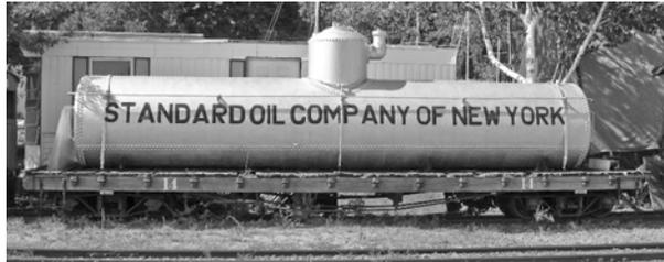
Car 22 at the Maine Narrow Gauge Museum was repainted into the Silver tank with the black Standard Oil lettering. It was painted with the number 14 on the flat car during our photography sessions which is incorrect as car 14 carried the larger tank which was made from individual panels which were riveted together.
