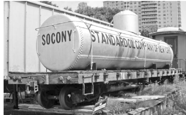
The brake wheel & staff normally would have been sticking up on this end of the car and placed just to the left of the draft gear.
