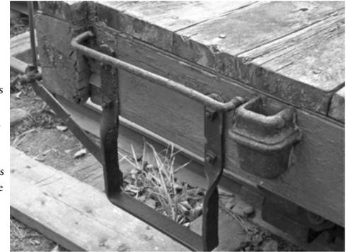
Each end of the flat car has an end step and a grab iron. The grab iron is wider than the end step.
